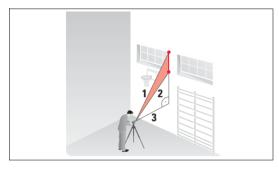
e.g. determining the height between point  ${\bf 1}$  and point  ${\bf 2}$  using three target points.
