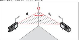
Press the key **two times** - the triangle symbol appears in the display.
