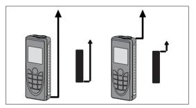
Press this button for **longer** the front reference is set permanently.
