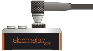
Figure 5. Transducer pressed against probe-disc
