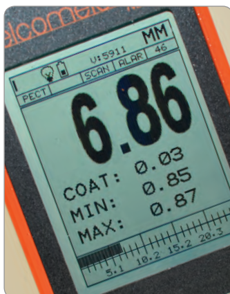
PECT mode on the CG100ABDL displaying material & coating thickness with scan bar
