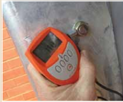
Zinc electroplating coating thickness 11.0µm.
