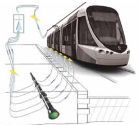
Figure 2: Stray voltage is the occurrence of electrical potential between two objects that ideally should not have any voltage difference between them.
