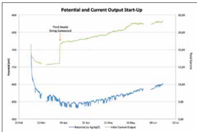
Potential and current output both started to increase about two weeks after CP start-up, which was surprising and a sign that there was a problem with the CP system.
