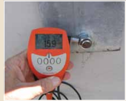
Zinc electroplating coating thickness 15.9µm.
