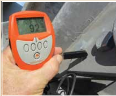
Zinc electroplating coating thickness 9.2µm.
