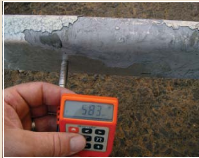
Thick coating – 583µm.
