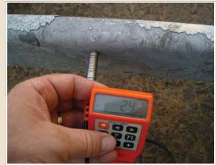
Very little (24µm) residual Fe/Zn alloy layer.
