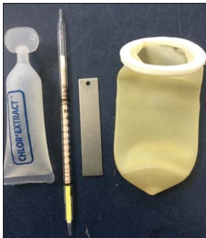
Sleeve test with Kitagawa tube.
