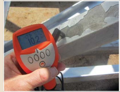
Very little (10.2µm) residual Fe/Zn alloy layer.
