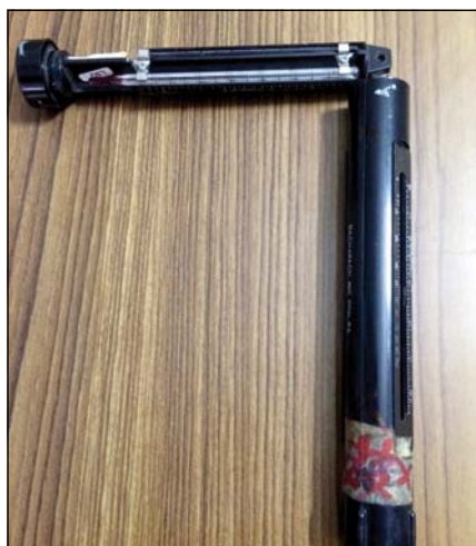
Sling psychrometer with two glass thermometers.
