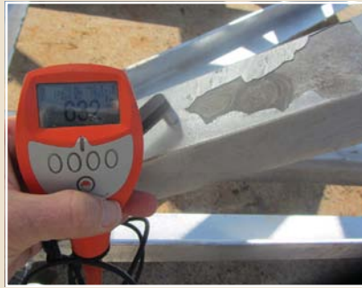
Thick coating – 632µm.
