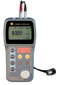
The new TIME TT2130 Ultrasonic Thickness Gauge / Material Thickness Gauge (previously TT300) is a handheld microprocessor-controlled thickness gauge, specifically designed for measuring the thickness of metallic and non-metallic materials eg. aluminium, titanium, plastics, ceramics, glass, cast iron and other good ultrasonic wave-conducting materials, as long as the material has parallel top and bottom surfaces.
