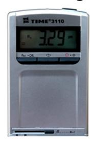
The TR3100 is a portable surface roughness tester. It has a large measuring range suitable for most materials and has Ra and Rz parameters. It features an external calibration at the keyboard. The TR3110 is equipped with a Li-ion Battery.
