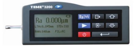
The TIME TR3200 / TR3202 Surface Roughness Tester (TR200) is a cost-effective roughness measuring instrument which supports a dozen of different parameters. It is small & light with high accuracy.
