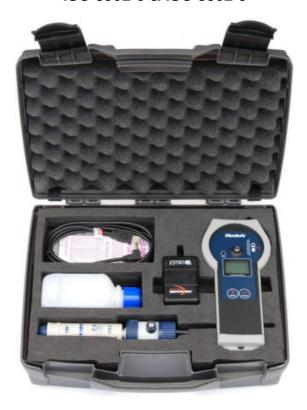
The Soluble Salt Meter (SSM) Salt Contamination Meter is developed specifically to address problems with US Navy and IMO test protocols using the Bresle Patch. The SSM exactly duplicates the Bresle Patch process but with a higher accuracy and reproducibility. Measurements are automated and there are no consumables. The complete test sequence requires less than a minute.
