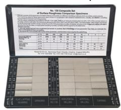
Comparators allow the estimation of surface roughness, by both touch and sight. This set consists of 30 comparison specimens, covering six commonly used and important machining methods:6 Turned, 6 End-Milled, 6 Horizontally Milled, 6 Ground, 3 Lapped, 3 Reamed / Drilled
