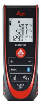
Now with Bluetooth®, a fully integrated intelligent endpiece, a bright white display and an ISO certified measuring engine that drives  $\pm$  1.5 mm accuracy and 100 metre measuring range. The Leica DISTO<sup>TM</sup> D2 is a 7 measurement mode LDM accurate to  $\pm$  1.5 mm. It features an intuitive back-lit LCD display in a 100g package that is small enough to fit in your pocket.
