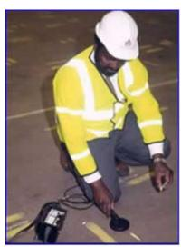
The Elcometer P120 Rebar Locator, is perhaps the easiest and fastest way of detecting reinforcing bars in concrete.
