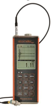
With a user selectable resolution of either 0.01mm or 0.001mm the PG70ABDL precision thickness gauge can display the thickness value together with A and B-Scan displays, providing users with the ability to accurately assess a wide range of materials.
