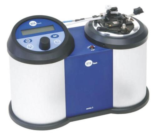
The Setaflash 'Series 3' Active-Cool Tester offers the same features as the Elcometer 6910/1 Setaflash but is fitted with a cup suitable for testing corrosive samples.
