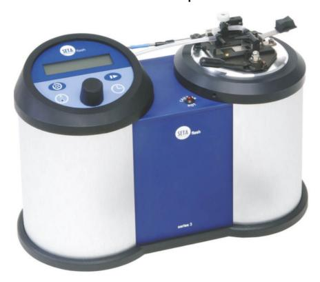
The Elcometer 6910/01 Closed Cup Tester is an easy to use instrument that can complete a flash/no flash test in less than two minutes or determine the flash point of a sample within a temperature range of ambient to 300°C
