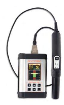
The **Elcometer 550** offers the user an unrivalled approach to measuring uncured powder thicknesses - **without touching the powder.** Traditional pre-cure powder thickness measurement requires contact with the coating however, the Elcometer 550 - using proven third generation ultrasonic technology - allows coating thickness measurements to be taken before the powder is cured and without touching the surface; allowing accurate prediction of the final coating thickness.
