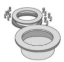
Disassemble the permeability cup
