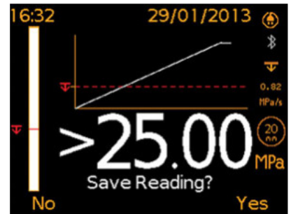
Individual user definable adhesion pull rate graphs can be saved with each reading.
