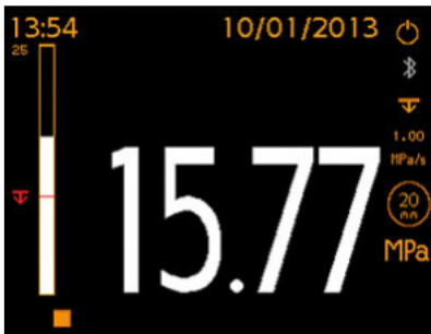
Automatic adhesion tester with selectable pull rates for 10, 14.2, 20 & 50mm diameter dollies.
