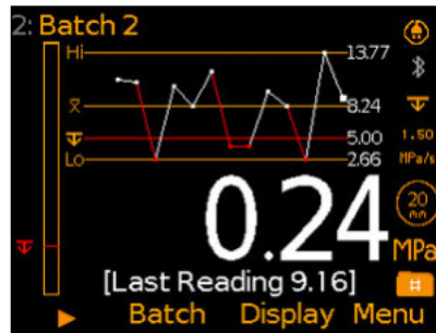
View adhesion trend graphs or live statistics alongside the reading value.
