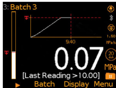
Either pull to maximum or pull to preset limit. Unique time hold feature allows users to set a delay before pressure returns to zero.
