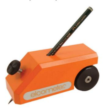
The pencil hardness test, also referred to as the Wolff-Wilborn test, uses the varying hardness values of graphite pencils to evaluate a coating's hardness.
