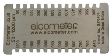
These stainless-steel combs are wire eroded to provide an accuracy  $\pm 5\%$  of marked value or  $\pm 3\mu$ m, whichever is greater, and are supplied with either Metric or Imperial measurements.
