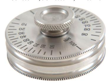
This instrument is similar to the Elcometer 3230 Wet Film Wheel, but is designed for use in the coil coating process.
