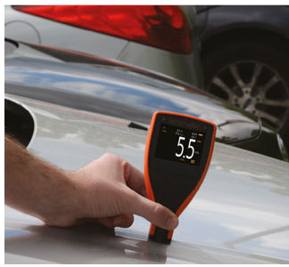
Measures on steel & aluminum body panels 1
