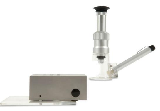
Measuring a coating's hardness using the indentation method, the Elcometer 3095 Buchholz Hardness Tester consists of a bevelled disc indenting tool which is fitted into a stainless steel block exerting a constant test load of 500g.
