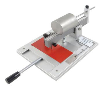
The Elcometer 3000 Manual Clemen Unit is a robust and simple to use instrument for evaluating the resistance to scratching of a coated surface.
