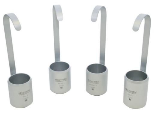
Thanks to its handle, the Elcometer Frikmar Viscosity Dip Cup is very easy to use to perform viscosity checks on site or during the manufacturing process.
