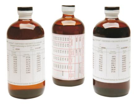
In order to check the viscosity cup's calibration or to certify it for ISO purposes, it is imperative that viscosity cup standard calibration oils are used.
