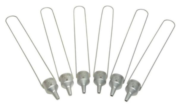
The Elcometer 2310 Shell Viscosity Dip Cups are stainless steel cups for quick measurements on-site or during production. These viscosity dip cups are often used in the printing or ink industry.
