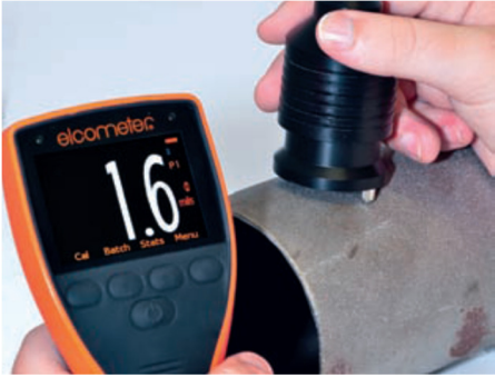
Integral or separate probes measure profiles up to 500 microns on flat or curved surfaces*
