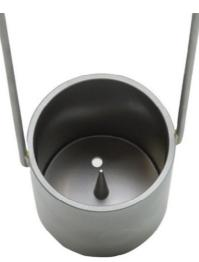
The Elcometer 2215 Lory Viscosity Cup is a conventional cylindrical cup with a needle fixed into the bottom for quick measurements on-site or during production.
