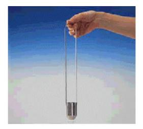
Easy-to-use stainless steel apparatus, for quick viscosity measurement of products on site or during production. The cup is first dipped into the product to be measured, then empties through the orifice.
