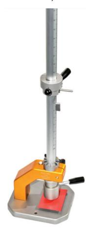
The Elcometer 1615 Variable Impact Tester is a simple to use gauge ideal for evaluating the resistance of a coating to impact (elongation, cracking or peeling).
