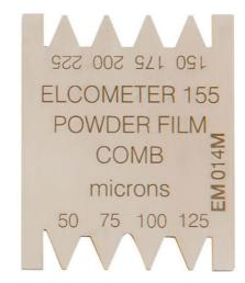
The Elcometer 155 is designed to measure uncured powder coating film thickness. This enables the application system to be set up and fine tuned prior to the curing process. In turn, this will reduce the amount of scrap and over-spray.
