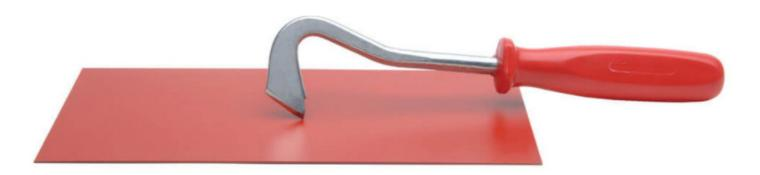
The Elcometer 1537 ISO Scratching Tool is a simple but effective instrument which is used to scratch the surface of samples in preparation for adhesion, salt spray and corrosion tests.
