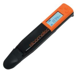
Incorporating a flat sensor, the Elcometer 138 Bresle Salt Meter measures the conductivity of a sample, then automatically converts this to show the density of salts, negating the need for the user to do a manual calculation when working in accordance with ISO 8502-6 or ISO 8502-9.
