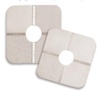
These extremely durable surface comparators allow the estimation of surface profile of either grit or shot blasted surfaces. Using the Elcometer 125 surface comparators as a reference the blasted profile can be compared to the four reference profile grades in each comparator. Profiles are recorded in microns. 4 Profile Values per Comparator.
