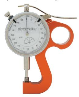
The proper and effective preparation of a surface prior to coating is essential. Making sure that the correct roughness – or profile – has been generated is essential. If the profile is too low, the adhesion of the coating to the surface will be reduced. Too high and there is the danger that the profile peaks will remain uncoated – allowing rust spots to occur.
