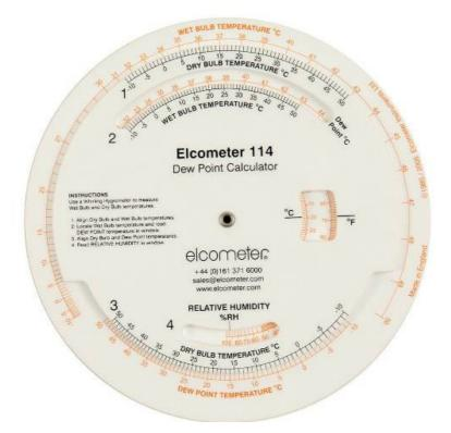
The Elcometer 114 Dewpoint Calculator provides accurate values of Dewpoint and Relative Humidity (RH) from the wet and dry bulb temperatures measured by a Whirling or Sling Hygrometer.
