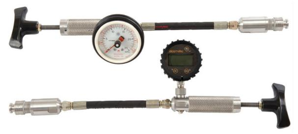
The Elcometer 108 Hydraulic Adhesion Tester is an extremely versatile Type III adhesion gauge which can be used for many adhesion requirements. Adhesion tests can be made on flat or curved (concave and convex) surfaces.
