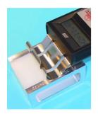
The test module PE30 is used for testing the accuracy of the DM4A moisture meter for wood and moisture measurements for building moisture measurements
