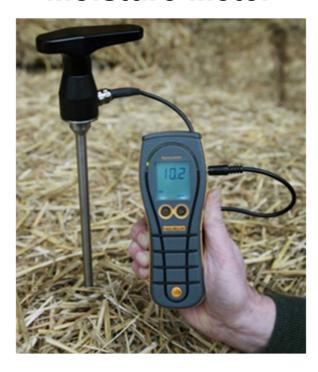
The Digital Balemaster (GRN 6165) is a hand held instrument which displays the results on a large LCD Digital Display. The probe is made from strong durable stainless steel and is 558mm long and 10mm in diameter, to reach the centre of big bales.
